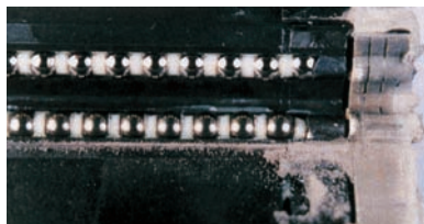
No foreign matter entering the raceway observed
