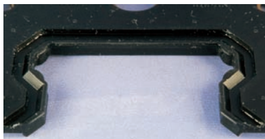
Lip has not been fractured
