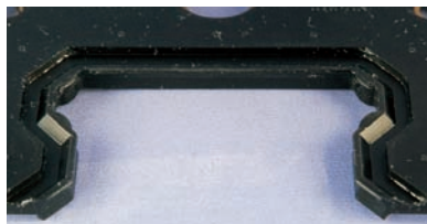
No. 2: with LaCS - no anomaly observed after traveling 5,000 km
